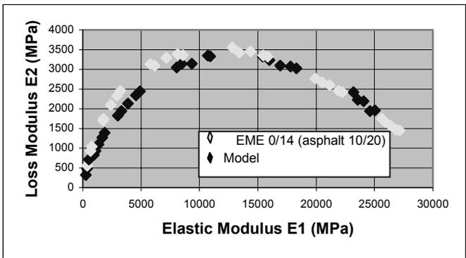
Figure 7. Rheological curves predicted by model and measured for EME 0/14 (High Modulus Mixture)
