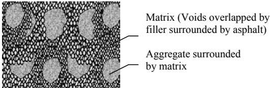
Figure 4. Structure supposed for HMA
