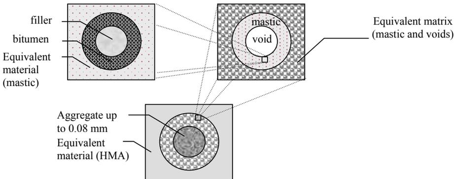
Figure 5. Representation of Hot Mix Asphalt by three spherical core-concentric shell model
