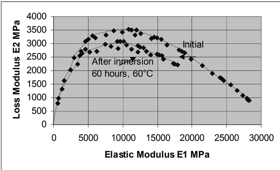
Figure 2. Variation in a Cole-Cole plot, after immersion (Mix B, Test -10 to 30°C)
