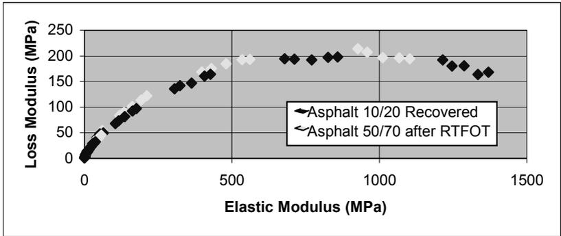
Figure 6. Rheological curves of two bitumen with different penetration grade
