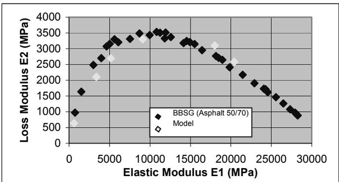
Figure 8. . Rheological curves predicted by model and measured for BBSG 0/10 (Mixture Dense)
