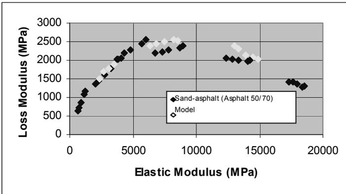
Figure 9. . Rheological curves predicted by model and measured for Sand-asphalt 0/6
