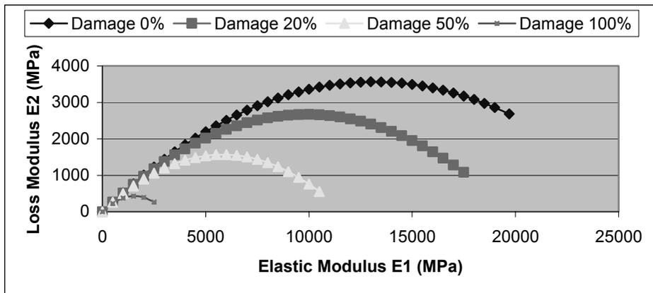
**Figure 11. Cole-Cole Plots of Moisture Damage**
