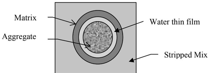
Figure 10. Model to Calculate Moisture Damage
