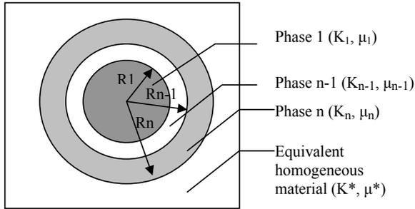
Figure 3. Spherical core-concentric shell model
