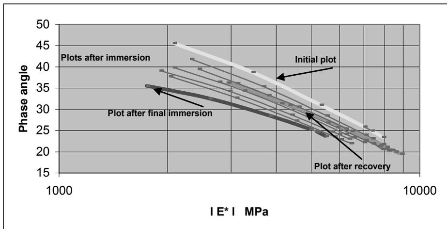
**Figure 1. Plots for bituminous mixtures in Black space with different immersion times (Mix A)**
