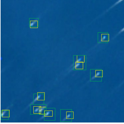
Fig. 11: Model struggles with close ship differentiation, generating a single bounding box for closely positioned vessels.
