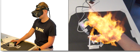
Figure 1: Participant wearing the VST-HMD, experiencing burning hands in VR and measuring the HPT.
