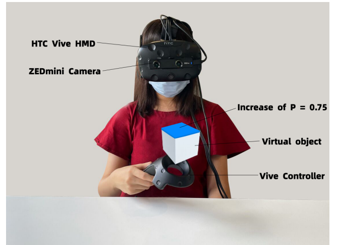
Figure 1: The user is holding a hand controller with a virtual object above it. The blue part in the cube is the 5.18% increment, denoted as the discrimination threshold's upper boundary.
