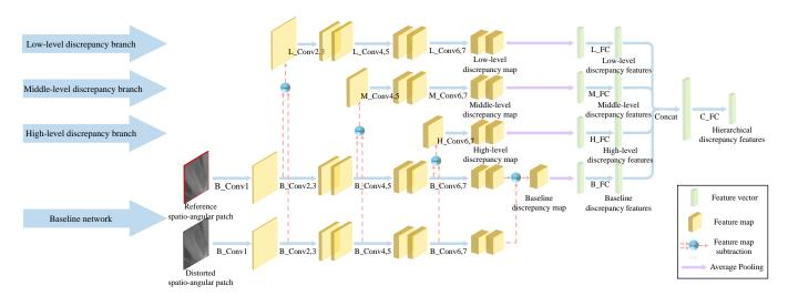
Fig. 4. Architecture of our proposed hierarchical discrepancy network, which consists of a baseline network and three discrepancy branches of different levels.
