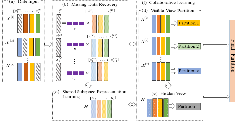
Fig. 2 Overview of CCIM-SLR. CCIM-SLR consists of six major components. (1) dotted module (a) represents the data input module; (2) dotted module (b) corresponds to the recovery of missing data through sparse low-rank techniques; (3) dotted module (c) focuses on shared subspace representation learning; (4) dotted module (d) stands for the partitioning module for the visible view; (5) dotted module (e) represents the partitioning module for the hidden view; (6) dotted module (f) signifies a collaborative learning partition module.
