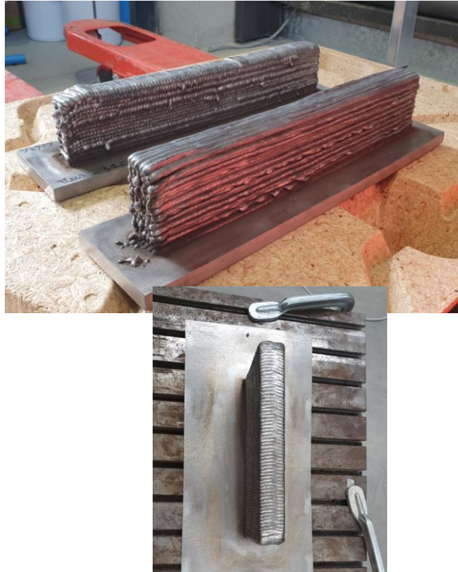
Fig. 1 Example of a part, obtained by WAAM process
