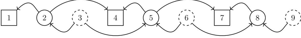
Fig. 7: Dependency graph for the application of  $A$ . Each circle/square is a task, i.e., the handling of one line of nodes. Tasks  $t^{(3k+1)}$ ,  $k = 0, 1, 2, \dots$  are within a square and are independent from all other tasks. An arrow from task  $t^{(i)}$  to task  $t^{(j)}$ , indicates that task  $t^{(i)}$  must wait for task  $t^{(j)}$  to finish.
