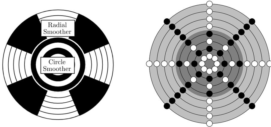
Fig. 3: **Left:** Schematic subdivision of a circular domain into an interior subdomain where circle-line smoothing is used and an exterior subdomain where radial smoothing is used. **Right:** Circular mesh with 64 nodes. Circular smoothing applied on the four interior circles (dark gray background color), radial smoothing applied on the four exterior circles (light gray background color). Nodes colored according to smoother color.
