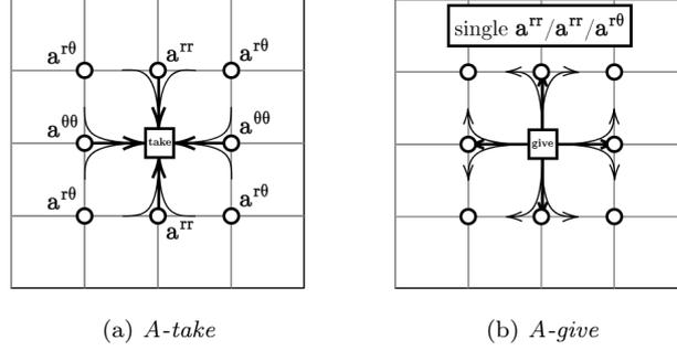
Fig. 5: Schematic representation of the two approaches to apply the matrix  $A$ : *take* or *give* the evaluations of the functions  $a^{xx}$  evaluations from or to the neighboring nodes, respectively.
