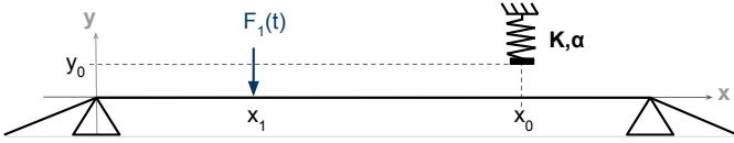
Fig. 1. Representation of the string configuration, as given in (1). An excitation force F_1 is applied at spatial coordinate x = x_1 , and an obstacle is located at (x_0, y_0) and modeled by a stiff non-linear spring, of stiffness K and nonlinear exponent \alpha .
