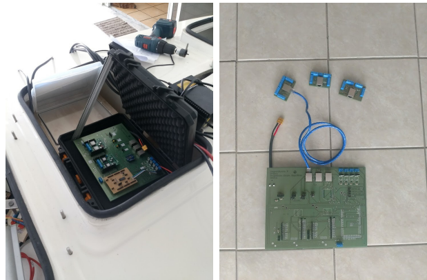
Fig. 6. Mother and slave boards specific developed and available for increasing components connectivity.
