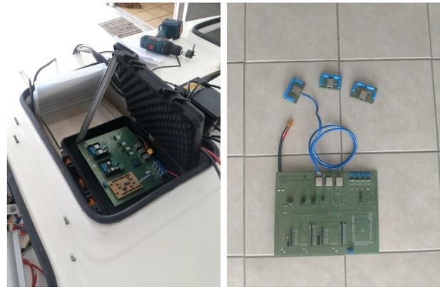
Fig. 6. Mother and slave boards specific developed and available for increasing components connectivity.
