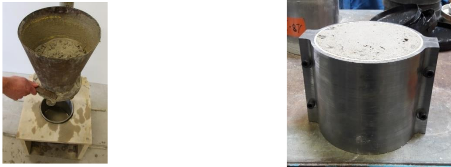
Figure 5 – Glanville apparatus for self levelling CLSM (left) and metallic counter-mold for compacted materials (right)
