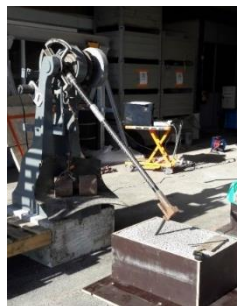
Figure 11 – Manual compaction of the trenches (left); mechanical excavation test (center); manual excavation test (right)
