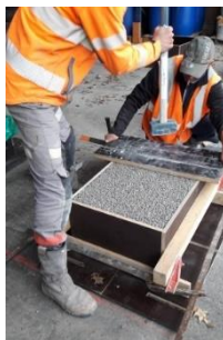
Figure 11 – Manual compaction of the trenches (left); mechanical excavation test (center); manual excavation test (right)
