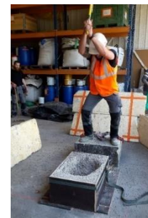
Figure 11 – Manual compaction of the trenches (left); mechanical excavation test (center); manual excavation test (right)
