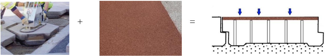
Figure 4: Principle of porous and draining RUP-FS slabs
