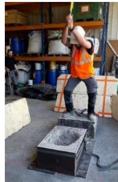
Figure 5 : Punching test in laboratory and manual pick excavation test
