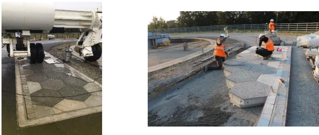
Figure 14 : Test on a RUP-SF prototype on the fatigue carousel available at Gustave Eiffel University
