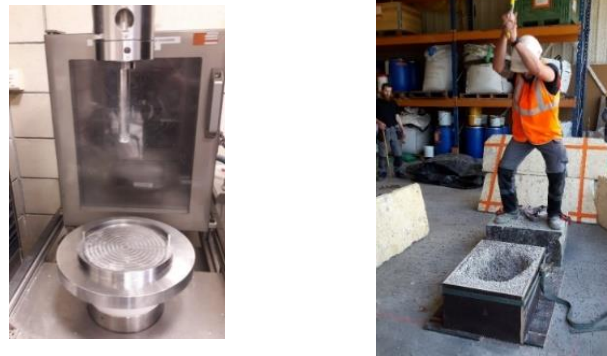
Figure 5 : Punching test in laboratory and manual pick excavation test
