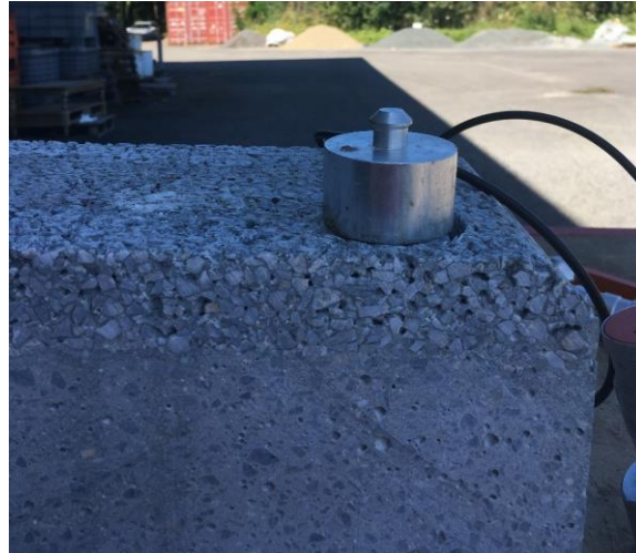
Figure 11 : Vertical section of a slab. The plain concrete interpenetrates partially the upper porous concrete layer. Metallic cylinder installed for pull-out test.
