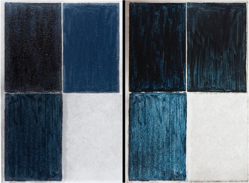
Fig. 71. Samples of indigo, diluted indigo (bottom left), azurite and unpainted alabaster. Left: frontal illumination and opaque background; right: the same samples when backlit.
