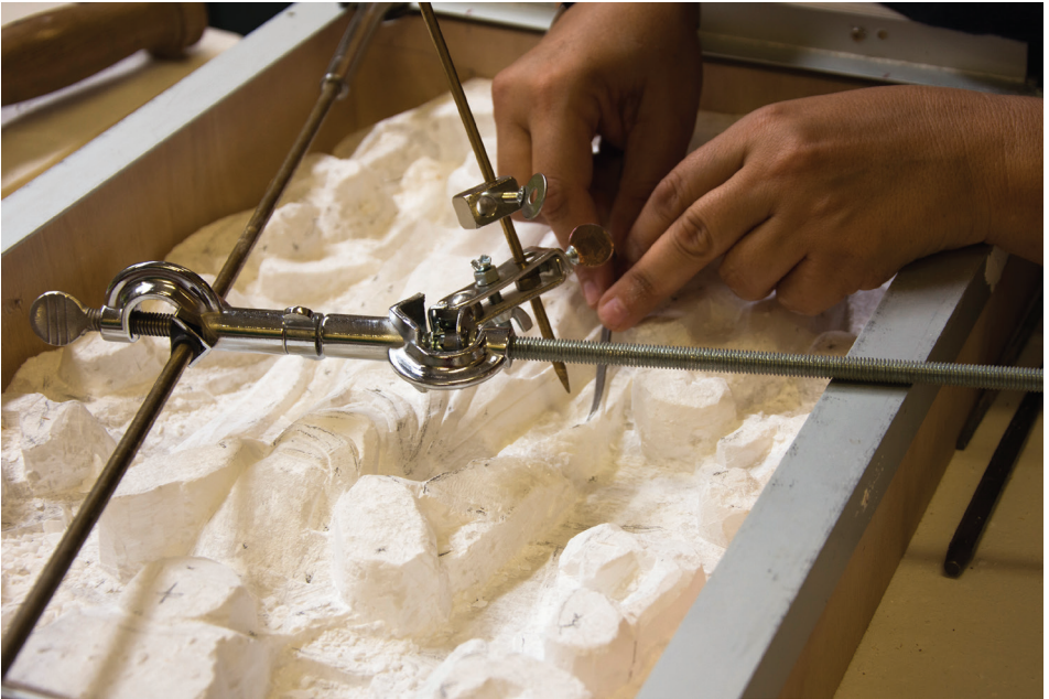
Fig. 54. Sculptor's pantograph (foreground) and digging with a riffler.
