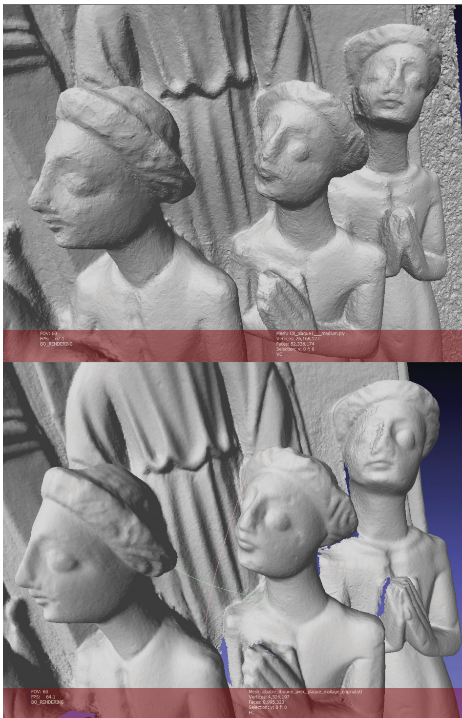
Fig. 7. Comparison between a photogrammetry (top) and a 3D scan (bottom). Libourne, Musée des Beaux-Arts, The Elect entering Paradise : detail of the Elect.
