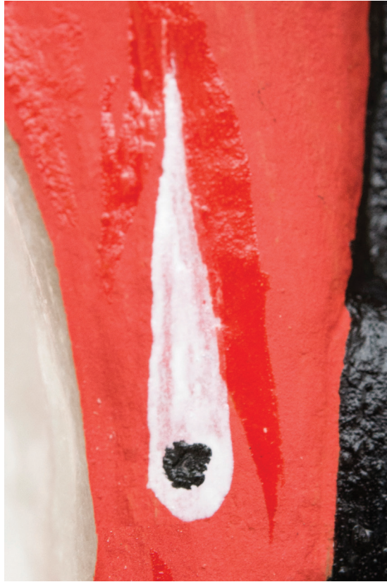
Fig. 65. Cinnabar applied in one layer (background) and two layers (around the white 'feather').
