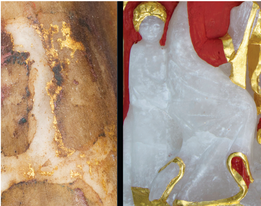
Fig. 13. Patinated alabaster. Bordeaux, cathedral, detail of the robe of the Virgin and Child (protected for a long time by gilding, the letter 'M' adorning the robe shows the original white polished surface; the surrounding areas are pitted and patinated). Right: Aspect of new alabaster: detail of a polished Spanish alabaster panel, carved and painted in 2018.
