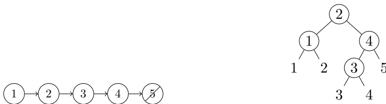
Figure 2: Left. A directed path on 5 vertices. Right. A possible strategy for the Regression Search Problem on the path on 5 vertices.
