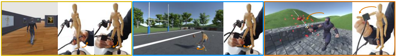
Figure 8: Examples of use cases (Left) Virtual visit: users move the prop's leg forward and backward to control a virtual walk. (Middle) Rugby kick: users shoot with the prop's leg. (Right) Sword slash: users move the prop's arm to cut virtual fruits.
