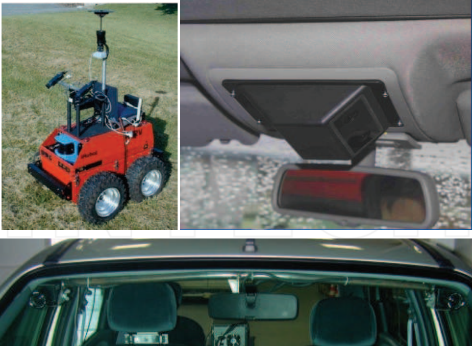
Fig. 1. Example of stereo setups, on a robot (top left) or inside a vehicle for cockpit monitoring (top right) or road perception (bottom)
