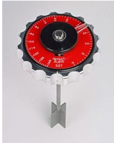
Figure 12: Photograph of a classic scissometer (Source: mtlabs.co.nz)
