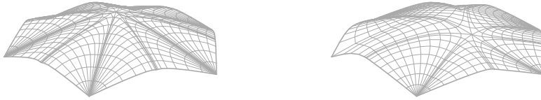
Fig. 10. Perspective views of the grid whose performances are compared for the different structural typologies: a symmetric topology with a central singularity (left) and an asymmetric topology with one singularity in the surface and two at corners (right).
