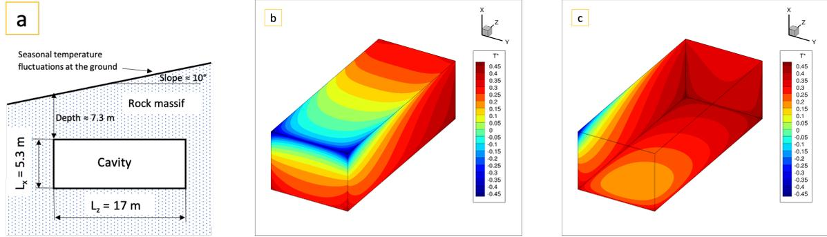
**Figure 1.** Geometry setup (a) and dimensionless temperature distribution (b and c) prescribed in the simulation and computed from a large-scale model [4] ( $Ra = 8.5 \times 10^9$ ).  $T^* = (T - T_0) / \Delta T$ .
