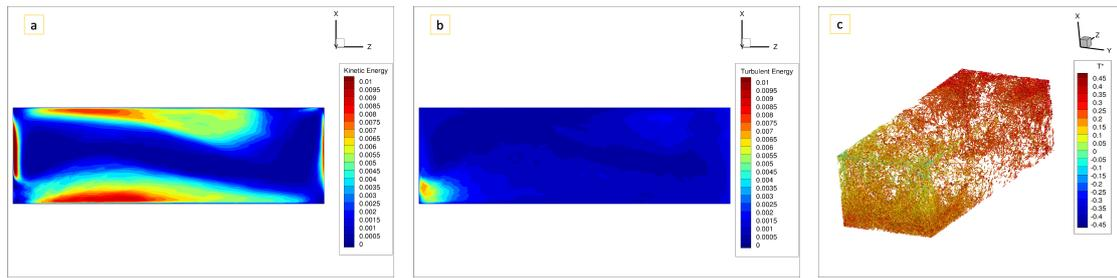
**Figure 2.** Kinetic energy of the mean flow  $\langle \bar{u}_i^* \rangle \langle \bar{u}_i^* \rangle / 2$  (a) and turbulent kinetic energy  $\langle \bar{u}_i^{*'} \bar{u}_i^{*'} \rangle / 2$  (b) in the  $y^*$  mid-plane. Where  $\langle . \rangle$  denotes the time average. Isosurfaces of the Q-criterion  $[\Omega_{ij}\Omega_{ij} - S_{ij}S_{ij}] / 2$  ( $Q = 10$ ) coloured by the temperature for an instantaneous flow field (c).
