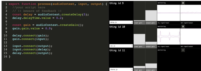
Fig. 4. The application interface in a web browser. On the left, a text editor to create and edit scripts in real time. On the right, different controls and monitoring for three devices connected to the application.
