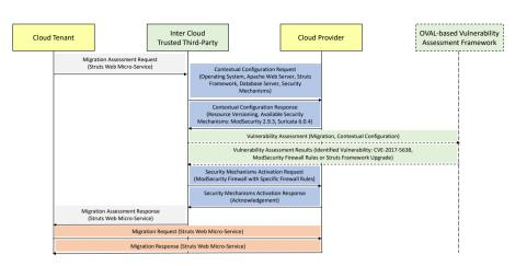
Fig. 3 Sequence diagram of the TOSCA-based interactions amongst the architectural building blocks
