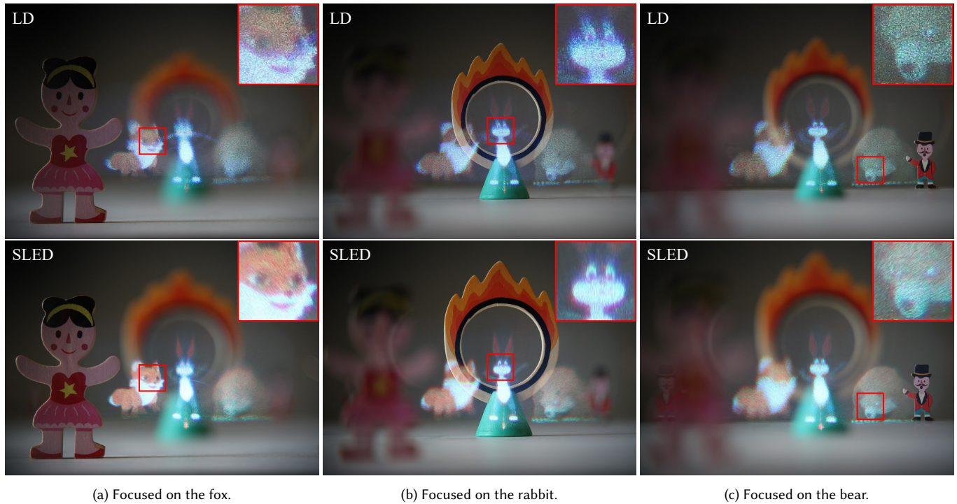
Fig. 9. Photographs captured through our prototype with a camera focusing on different depths, using the LD (top row) and SLED modules (bottom row). When the camera is focusing on a given 3D model, the corresponding real-world object is also focused while other parts of the scene appear blurred, demonstrating that our proposed holographic AR headset provides accurate accommodation depth cues. Compared to LDs, the SLED module significantly reduce speckle noise artifacts while preserving the sharpness of in-focus regions in the reconstructed images (see supplementary video).
