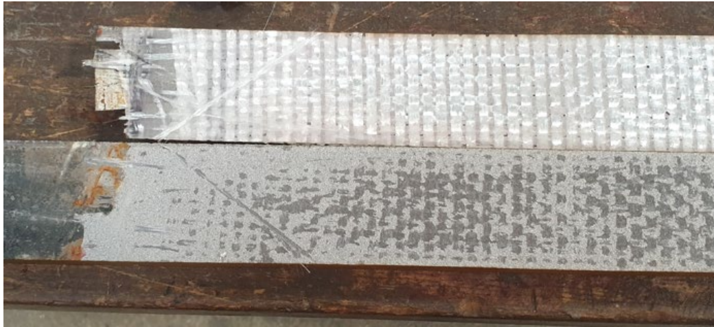
Figure 12. Fracture surfaces of the fatigue test samples in tension.
