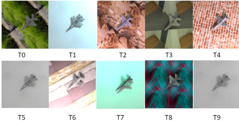
Figure 3: There are 10 tasks in our benchmark, T_i represents the i -th task. The difference between tasks is the background and illumination. T_5 correspond to the original Jacquard dataset. T_0, T_2, T_3, T_4, T_6, T_8 use a different background. T_1, T_7 use a different illumination. In T_9 , we apply a gaussian filter to blur the input image.
