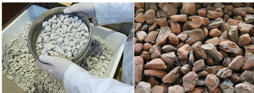
Figure 1. Materials used for biogas desulfurization. (Left) Cellular concrete (CC). (Right) Expanded schist (ES).
