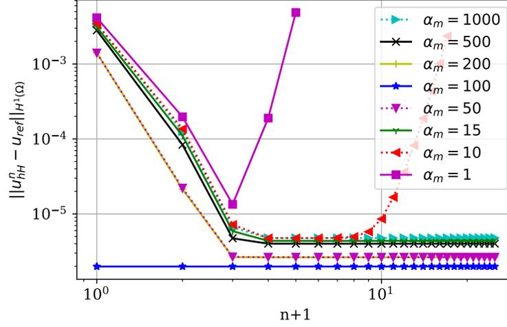
Figure 6: The relative error in  $H^1(\Omega)$ -norm with respect to the variation of the number of iteration  $n$  for different values of contrast between  $\alpha_m$  and  $\alpha_f = 100$ , non-matching meshes ( $h = \frac{L}{120}, H = \frac{L}{40}$ ) and a non-conformal macro mesh with the inclusion  $\partial\Omega_f$ .
