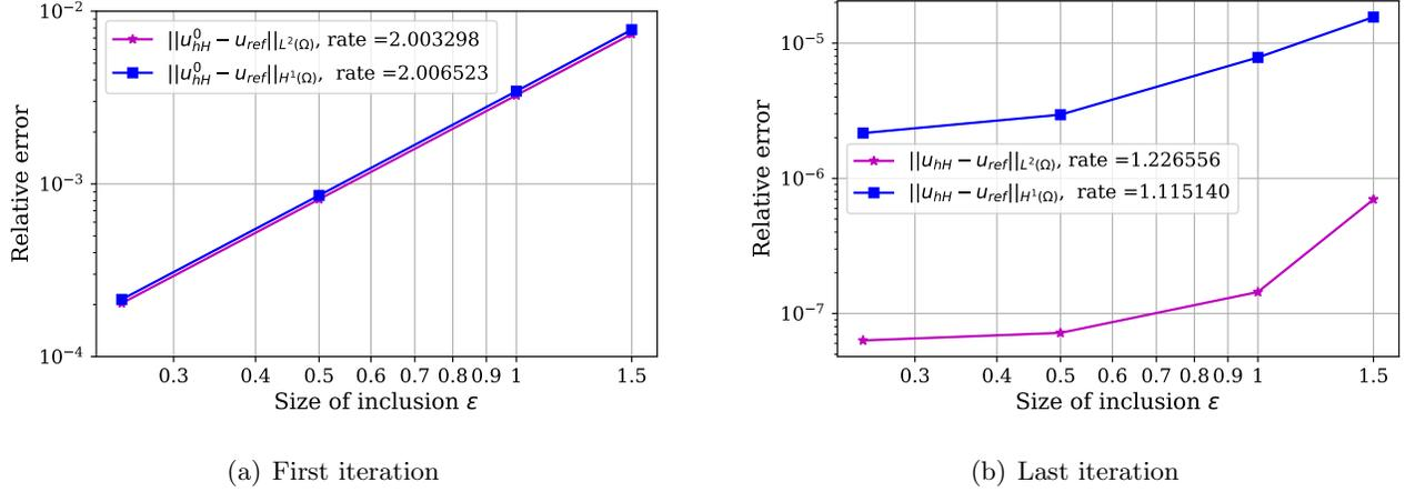
Figure 10: The relative error in  $L^2(\Omega)$  and  $H^1(\Omega)$  norms according to the size of the inclusion  $\varepsilon$  with a non-conformal mesh with the macro model boundary  $\partial\Omega_f$ .
