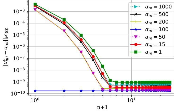
Figure 5: The relative error in  $H^1(\Omega)$ -norm for different values of contrast (between  $\alpha_m$  and  $\alpha_f = 100$ ) and with the same mesh for the reference, micro and macro model ( $h = H = h_{\text{ref}} = \frac{L}{40}$ ).
