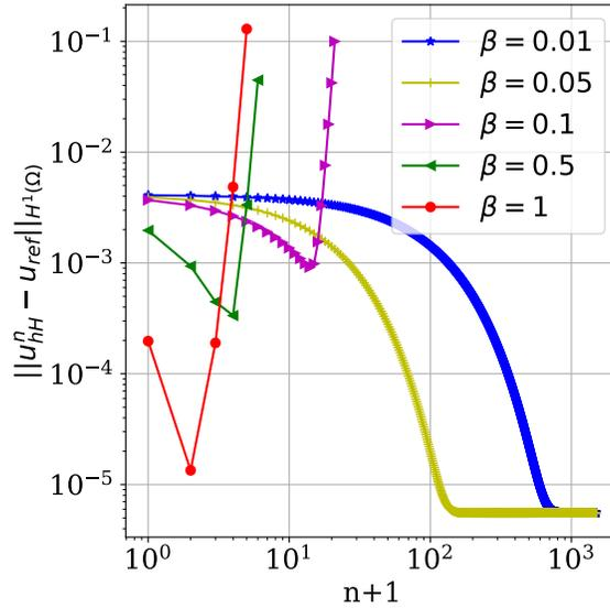
Figure 8: The relative error in  $H^1(\Omega)$ -norm with respect to the variation of the number of iteration  $n$  for different values of the relaxation coefficient (with  $\alpha_m = 1$  and  $\alpha_f = 100$ ), non-matching meshes ( $h = \frac{L}{120}$ ,  $H = \frac{L}{40}$ ) and a non-conformal macro mesh with the inclusion  $\partial\Omega_f$ .
