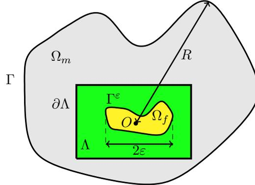
Figure 1: A small inclusion in an elastic medium
