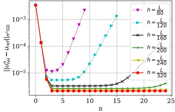
Figure 7: The relative error in  $H^1(\Omega)$ -norm with respect to the variation of the number of iteration  $n$  for different values of micro-mesh size (with  $\alpha_m = 10$  and  $\alpha_f = 100$ ), non-matching meshes ( $H = \frac{L}{40}$ ) and a non-conformal macro mesh with the inclusion  $\partial\Omega_f$ .
