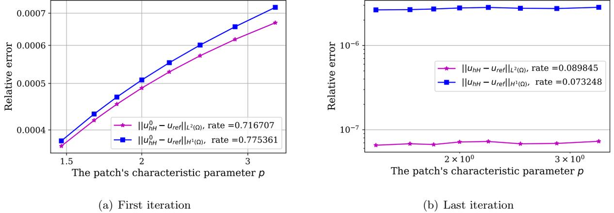
Figure 9: The relative error in  $L^2(\Omega)$  and  $H^1(\Omega)$  norms for the first and last iteration of the iterative method with respect to the patch characteristic parameter  $p$  with  $h = \frac{L}{80}$ ,  $H = \frac{L}{40}$  and a non-conformal mesh with the macro model boundary  $\partial\Omega_f$ .
