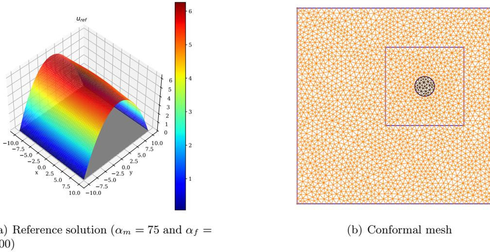
Figure 3: A reference solution and an example of a conformal mesh with  $h_{\text{ref}} = \frac{L}{20}$
