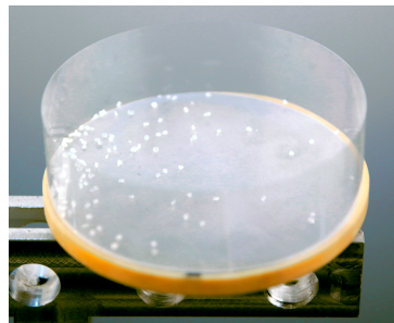
Figure 1. Salt grains bouncing over a vibrated rigid disk (radius 9 cm). The vibration amplitude increases from left to right.
