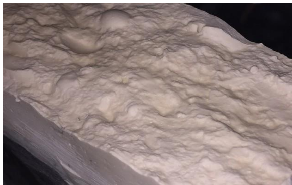
Fig. 3 Realistic crack surface relief after complete opening of the specimen.
