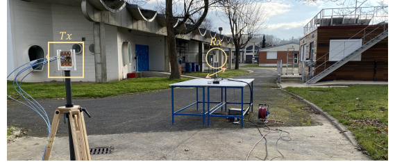
Fig. 3. FDA-SDF outdoor measurement setup.
