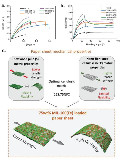
Figure 4. a) Strain-stress curves of 75 wt.% nano-MIL-100(Fe) paper sheets made with different cellulosic matrices. b) Force versus angular deflection of the paper sheets containing different cellulosic matrix investigated by two-point method to deduce the flexibility of the 75 wt.% nano-MIL-100(Fe) paper sheets. c) Scheme highlighting the benefits of combining two different cellulosic matrices to produce a paper sheet consisting of 75 wt.% MIL-100(Fe) with good mechanical properties.
