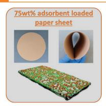
A green one-pot route combining two cellulosic products of different dimensions to prepare high-loading (>70 wt.%) porous solids (metal–organic frameworks, carbons, zeolites) paper sheets, with good flexural and strength mechanical resistance and preserved adsorption properties.
