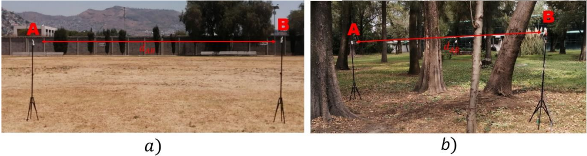
Fig. 1 Two different scenarios with LOS conditions: a) open scenario free of obstacles, b) semi-forest scenario with some trees around.
