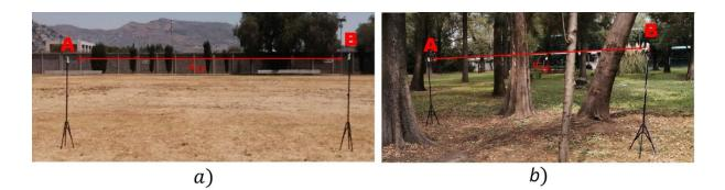
Fig. 1 Two different scenarios with LOS conditions: a) open scenario free of obstacles, b) semi-forest scenario with some trees around.
