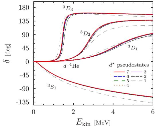
FIG. 1. (Color online) Computed  $d$ - ${}^4\text{He}$   $S$ - and  $D$ -wave phase shifts at  $N_{\text{max}} = 8$  and  $\hbar\Omega = 20$  MeV, obtained with fifteen square-integrable  ${}^6\text{Li}$  eigenstates and up to seven  ${}^2\text{H}$  pseudostates in each of the  ${}^3S_1$ - ${}^3D_1$ ,  ${}^3D_2$  and  ${}^3D_3$ - ${}^3G_3$  channels. The two-body part of the SRG-evolved  $\text{N}^3\text{LO}$   $NN$  potential ( $NN$ -only) with  $\Lambda = 2.0 \text{ fm}^{-1}$  was used.
