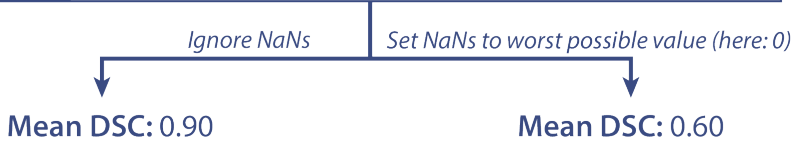
Extended Data Fig. SN 2.31. Effect of invalid predictions (missing values) when aggregating metric values. In this example, ignoring missing values leads to a substantially higher Dice Similarity Coefficient (DSC) compared to setting missing values to the worst possible value (here: 0).
