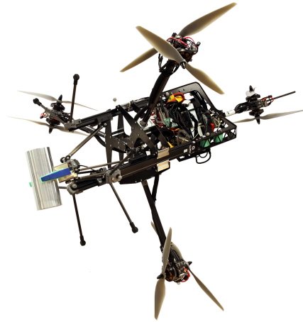
Fig. 1. PrisMAV , the integrated aerial manipulator with a linear delta arm.
