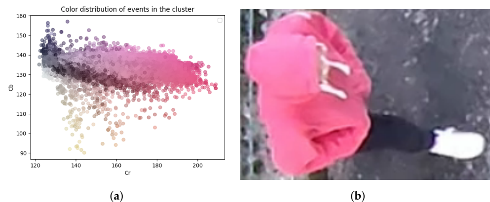
Figure 9. Color scattering for Pedestrian : (a) scatter plot, with each point corresponding to an event; (b) exemplary content of the cluster.
