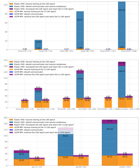
Figure 5: Costs (seconds) of recovering/reconfiguring workers when training the VGG-16 model in three scenarios: Scenario I: Dropping the failed process/node ("Down"); Scenario II: Remaining the original worker size by replacing the failed process/node with new process/node ("Same"); Scenario III: Automated doubling the worker size during the training ("Up"); scaling from 12 GPUs to utmost 192 GPUs
