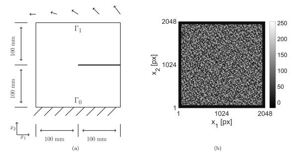
Figure 10: Large-sample experiment. Geometry of the sample and applied boundary conditions (a), speckle pattern applied to the sample surface (b). The pixel size is  $104 \mu m$ .
