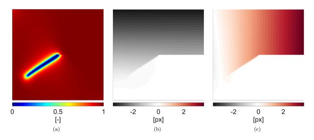
Figure 11: Solution of the phase-field model of the large-sample test at frame 75 for the reference parameters. Phase-field variable  $\varphi$  (a), displacements  $u_1$  (b) and  $u_2$  (c).
