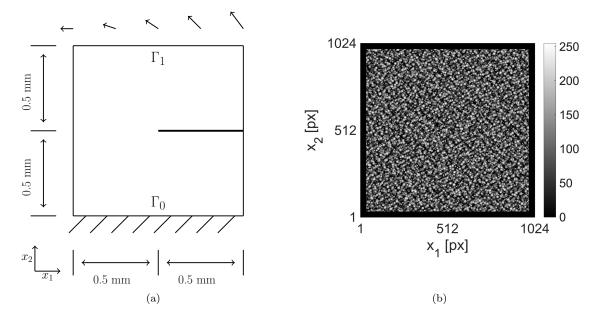
Figure 1: Small-sample experiment. Geometry of the sample and applied boundary conditions (a), speckle pattern applied to the sample surface (b). The pixel size is about 1 µm.
