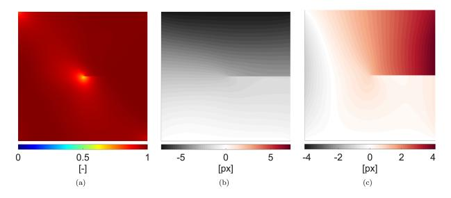
Figure 3: Solution of the phase-field model of the small-sample test at frame 75 for the initial parameterization  $p^{(0)}$ . Phase-field variable  $\varphi$  (a), displacements  $u_1$  (b) and  $u_2$  (c).
