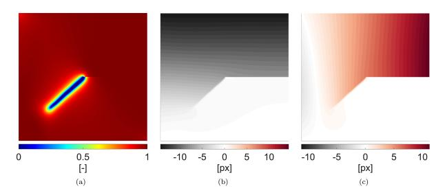
The crack starts propagating from the beginning of the slit at frame 43 toward the bottom/left corner.
