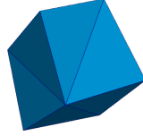
Figure 5. Example of randomly perturbed Cartesian cell with non planar faces cut into two triangles
