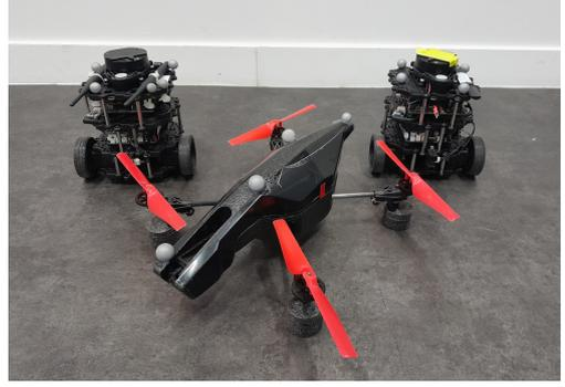
Fig. 2: Ground and aerial robots used in the cooperation system.
