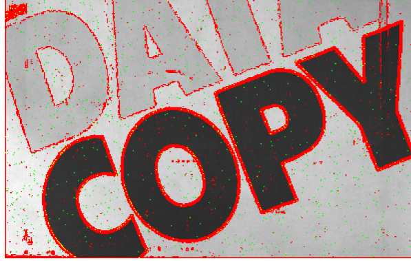
Figure 3. The error map obtained by combining the redundancy criterion and the intensity variation detector. The intensity is displayed in gray level, the redundancy criterion based detector in green and the intensity variation detection in red. In yellow appear the pixels detected by both detectors as problematic.
