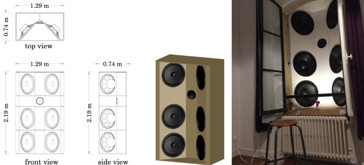
Figure 4. Cabinet design. Left drawings: installation of the loudspeaker, six subwoofers and their back volumes (top, front, side and 3D views). Right photograph: simulator viewed from inside the bedroom.
