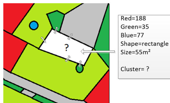
Figure 3. Illustration of the MRF clustering problem with very few features: in this example, we try to guess the cluster of the central segment based on five features and the clusters of its neighbor segments (identified using the colors).
