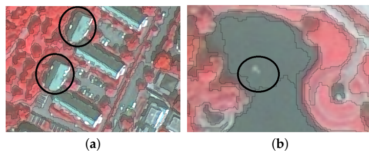
Figure 2. Examples of over-segmentation and under-segmentation. (a) Example of an over-segmentation on two houses that could be fixed during the clustering step: the algorithm may still detect that these two segments are part of the same cluster; (b) example of an under-segmentation where the white object in the middle of the lake was not detected during the segmentation step and will never be since it is now merged with a lake segment.
