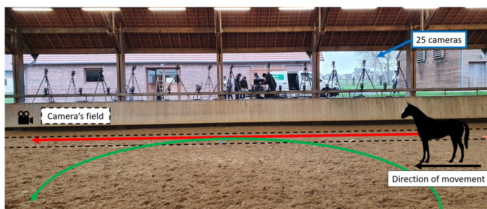
Figure 2. Positioning of the Vicon cameras on one side of the indoor arena. The black dotted lines correspond to the camera's field. The trajectory of the straight line during walking and trotting is represented by the red arrow, and the trajectory of the circle during galloping is represented by the green arrow.
