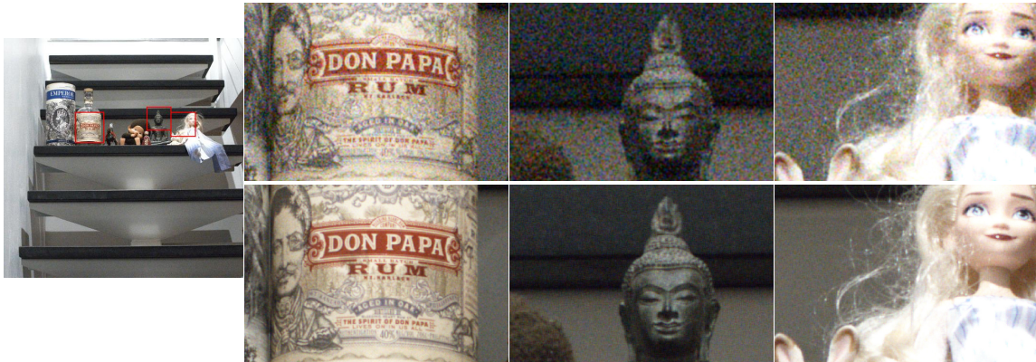
Figure 15. burst super-resolution on real raw bursts exploiting our alignment method. Top: low-resolution crops. Bottom: super-resolution exploiting our alignment method. Data kindly provided by the authors of [28]. It is best seen by zooming aggressively on a computer screen.
