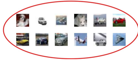
Figure 1. Example of bag sample created from CIFAR10 [12]. The positive target class is dogs, and the negative classes are planes and cars. The bag is labeled as positive as it contains two instances of dogs.
