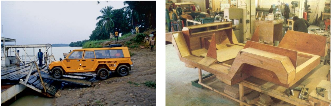
Figure 60: One of the 3 Africars crossing the Ubangui River and a plywood chassis [230].
