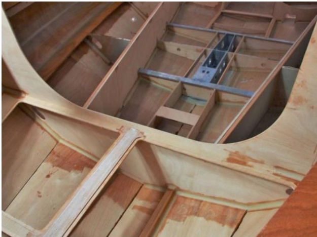
Figure 55: Plywood structure of an RM sailboat [219]
