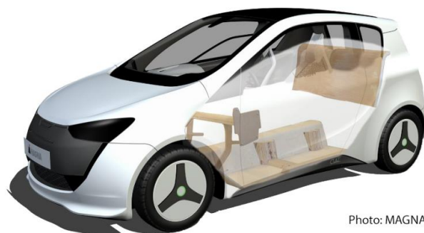
Figure 63: (a) wood frame on a snow mobile; (b) Wood part on CULT Car project (Reproduced from [237]).
